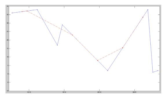
In this figure, the blue line represents the original data values while the red line represents the resampled data at a new set of timestamps. These new timestamps are marked by red stars while the original timestamps are marked by blue circles.
