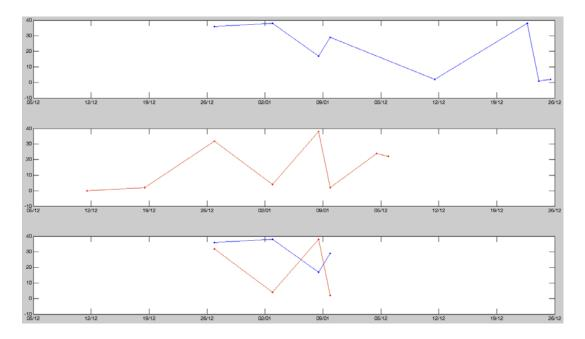
The previous figure shows how the values of two data objects, plotted in the first and second positions respectively, can be intersected to produce a new object whose elements contain only timestamps common to the original two. Uncommon timestamps are discarded along with their data values.
