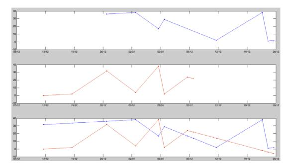
The top two plots above depict two separate data objects. The bottom plot is the result of these two data objects being passed to the tsunion function. You can see that in the bottom plot that each element has been extended to include the timestamps of the other and that values have been extrapolated to satisfy these new timestamps.
